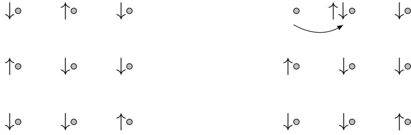
Fig. 4: For U/t \gg 1 , the cost of a hopping is E(|\uparrow\downarrow\rangle) + E(|0\rangle) - 2E(|\uparrow\rangle) = U
