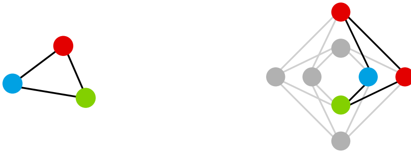
Fig. 15: A graph with triangular connectivity (left) can be mapped onto the Chimera hardware graph (right) by using two physical qubits for one of the logical qubits.
