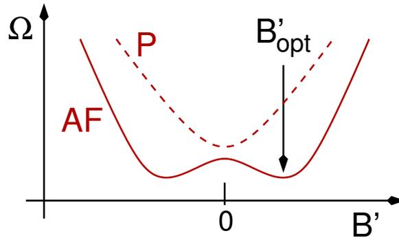
**Fig. 2:** Grand potential  $\Omega$  as a function of a Weiss field  $B'$  in the case of a paramagnet (P) and in the case of an antiferromagnet (AF).  $B'$  is a fictitious staggered field, the optimal value of which ( $B'_{\text{opt}}$ ) must be determined by minimization of  $\Omega$ . As there is no physically applied staggered field, i.e.  $B = 0$ , a finite  $B'_{\text{opt}}$  indicates spontaneous symmetry breaking.
