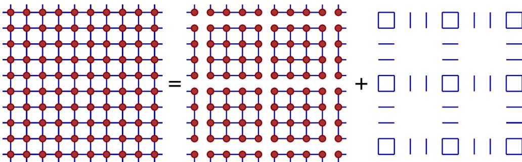
**Fig. 1:** Sketch of the decomposition of the original system  $H = H_0(\mathbf{t}) + H_1$  into a reference system  $H' = H_0(\mathbf{t}') + H_1$  and the inter-cluster hopping  $H_0(\mathbf{V})$  for a square lattice and cluster size  $L_c = 16$ . Blue lines: nearest-neighbor hopping  $t$ . Red dots: on-site Hubbard interaction.
