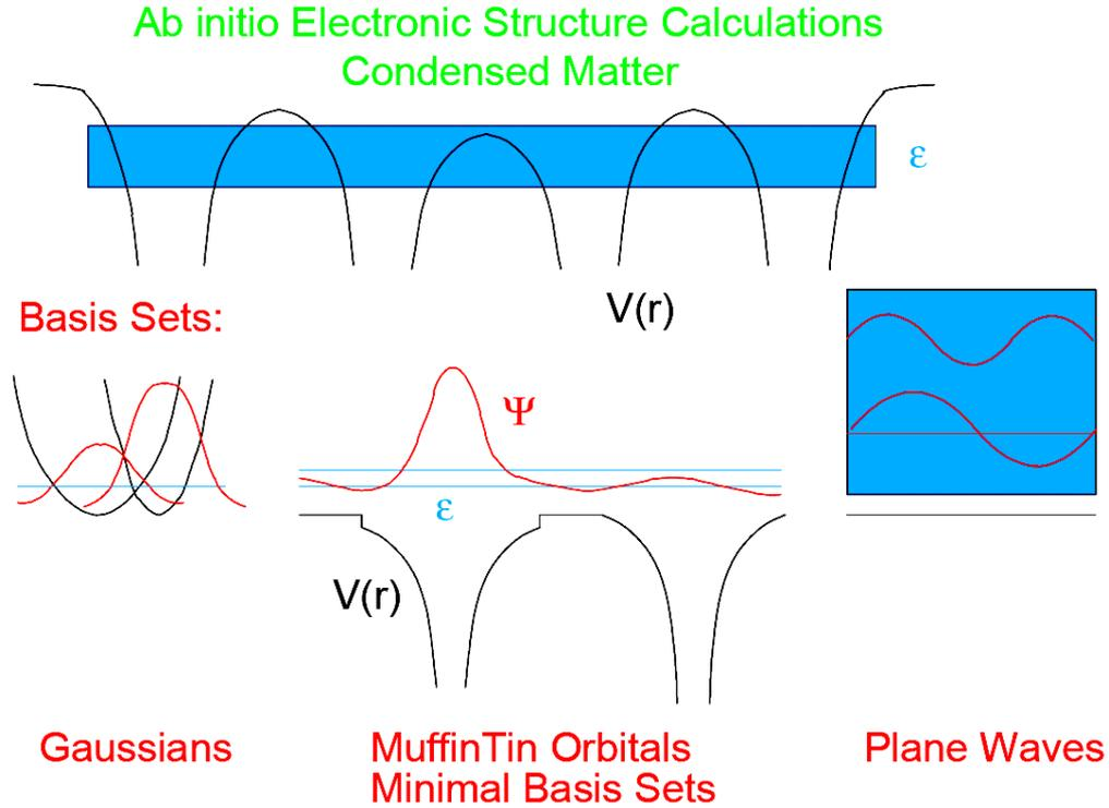
**Fig. 1:** Top: Effective one-electron potential in condensed matter (black) and the energy region of interest (blue). Bottom: Basis functions (red), their generating potentials (black), and energies (blue).
